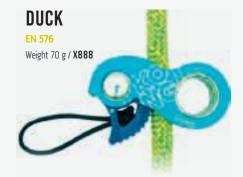
Duck - a new rope clamp/positioner made by Kong, designed for ropes with diameters between 8 and 13 mm. The first and only device that may be used also with 10 to 15 mm wide flat and tubular slings. Due to its small dimensions, it is possible to use Duck with one hand only, the large diameter enables the karabiner to rotate. Intended for ascending activities, daisy chain positioning, self-belaying.
