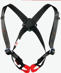
Chest harness SCOUT must be used in combination with a sit harness. It has two buckles for adjustment purposes and the height of attachment may be selected according to its position.
