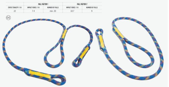
DynaProt 10, the dynamic sling, is made of a dynamic rope and is therefore capable of absorbing the energy of a dynamic fall and to dampen this fall thanks to its elongation. DynaProt 10 has been tested with fall factors 1 and 2. It is able to arrest nine falls with a fall factor of 2. Even with a fall factor of 2, the impact force is lower than the maximum force permitted by EN 892.
